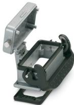
Panel mounting base B16, with single locking latch, material: die-cast aluminum, protective cover material: Al, height: 29 mm, cable gland: none, protective cover: yes, Standard, with flat gasket
