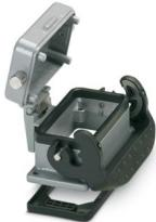
Panel mounting base B10, with single locking latch, material: die-cast aluminum, protective cover material: Al, height: 29 mm, cable gland: none, protective cover: yes, Standard, with flat gasket
