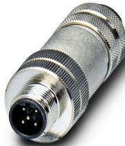
Data connector, PROFIBUS, INTERBUS, 5-position, shielded, Plug straight M12, coding: B, Screw connection, knurl material: Zinc die-cast, nickel-plated, cable gland Pg9, external cable diameter 6.5 mm ... 8.5 mm
