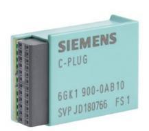
C-plug, removable data storage medium For simple device replacement in case of fault, for recording configuration or engineering and application data, can be used in the following SIMATIC NET products with C-plug slot: SCALANCE XC-200, XP-200, XM-400, XR-500, M-800, W-700, SC-600 and S615.
