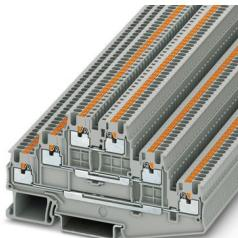
Multi-level terminal block, nom. voltage: 500 V, nominal current: 15 A, connection method: Push-in connection, 1 level, Rated cross section: 1.5 mm<sup>2</sup>, cross section: 0.14 mm<sup>2</sup> - 1.5 mm<sup>2</sup>, mounting type: NS 35/7,5, NS 35/15, color: gray
