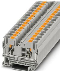
Feed-through terminal block, nom. voltage: 1000 V, nominal current: 41 A, number of connections: 2, number of positions: 1, connection method: Push-in connection, Rated cross section: 6 mm<sup>2</sup>, cross section: 0.5 mm<sup>2</sup> - 10 mm<sup>2</sup>, mounting type: NS 35/7,5, NS 35/15, color: gray
