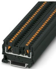
Feed-through terminal block, nom. voltage: 800 V, nominal current: 32 A, number of connections: 2, connection method: Push-in connection, Rated cross section: 4 mm<sup>2</sup>, cross section: 0.2 mm<sup>2</sup> - 6 mm<sup>2</sup>, mounting type: NS 35/7,5, NS 35/15, color: black
