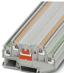
Double-level terminal block, nom. voltage: 400 V, nominal current: 9 A, number of connections: 4, connection method: Push-in connection, 1st and 2nd level, Rated cross section: 1.5 mm<sup>2</sup>, cross section: 0.14 mm<sup>2</sup> - 1.5 mm<sup>2</sup>, mounting type: NS 35/7,5, NS 35/15, color: gray
