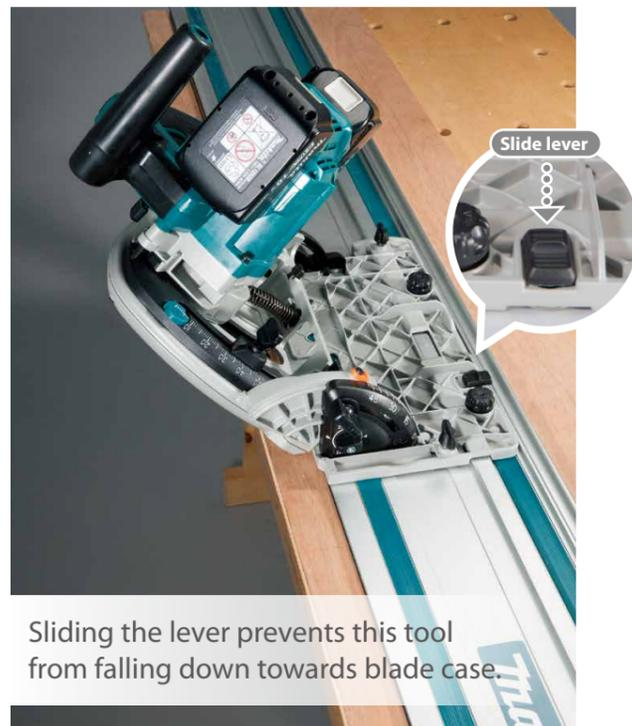
Sliding the lever prevents this tool from falling down towards blade case.
