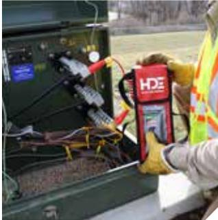
Visual Indication of Open Circuits, Short Circuits, Shorted Turns or Windings
