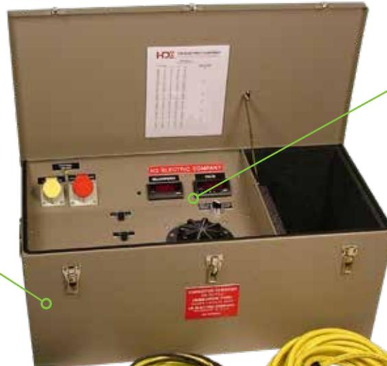
Meters Display Current Through Each Capacitor and Voltage Applied to Capacitor Bank
