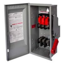
Siemens Low Voltage Circuit Protection Heavy Duty Safety Switch. 3-Pole 3-Wire Fused in a type 12 industrial enclosure. Rated 600VAC (100A). Special features: Crouse-Hinds interlocked receptacle, viewing window.
