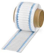
Shrink sleeve, Roll, white, unlabeled, can be labeled with: THERMOMARK E.300 (D)/600 (D), THERMOMARK ROLLMASTER 300/600, THERMOMARK ROLL X1, THERMOMARK ROLL, THERMOMARK ROLL 2.0, THERMOMARK W, THERMOMARK X1.2, perforated, mounting type: slide-on, cable diameter range: 1 ... 3.2 mm, lettering field size: 30 x 5 mm, Number of individual labels: 2000
