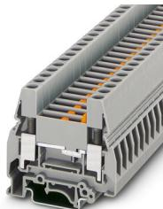
Test disconnect terminal block, nom. voltage: 500 V, nominal current: 57 A, connection method: Screw connection, Rated cross section: 10 mm<sup>2</sup>, cross section: 0.5 mm<sup>2</sup> - 16 mm<sup>2</sup>, mounting type: NS 35/7,5, NS 35/15, NS 32, color: gray
