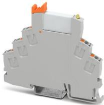
Preassembled relay module with Push-in connection, consisting of: relay base with ejector and power contact relay. Contact switching type: 1 changeover contact. Input voltage: 24 V DC
