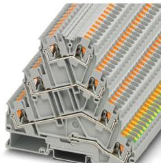
Motor terminal block, four-level, connection method: push-in connection, cross section: 0.2 mm<sup>2</sup> - 6 mm<sup>2</sup>, AWG: 24 - 10, width: 6.2 mm, height: 95.4 mm, color: gray, mounting type: NS 35/7,5, NS 35/15
