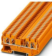
Feed-through terminal block, nom. voltage: 800 V, nominal current: 32 A, number of connections: 4, connection method: Push-in connection, Rated cross section: 4 mm<sup>2</sup>, cross section: 0.2 mm<sup>2</sup> - 6 mm<sup>2</sup>, mounting type: NS 35/7,5, NS 35/15, color: orange
