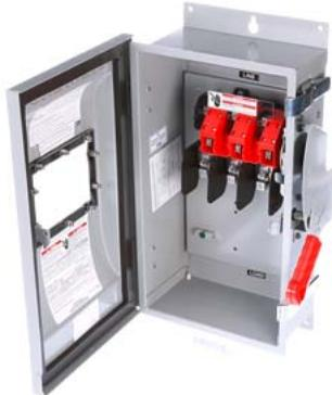
Siemens Low Voltage Circuit Protection Heavy Duty Safety Switches. Type: ENCLOSED, SAFETY SWITCH Std: CSA V. Rating: 600V A. Rating: 30 A Wattage: 3W No. Of Poles: 3P F. Rating: 60Hz Action: SINGLE THROW Material: 304SS Enclosure: TYPE 12. 2-3 point mounting holes. Insulation: YES O. Cycles: 10000 O. Temperature: (-20F-120F) AMBIENT TEMPERATURE Environmental Conditions: INDUSTRIAL
