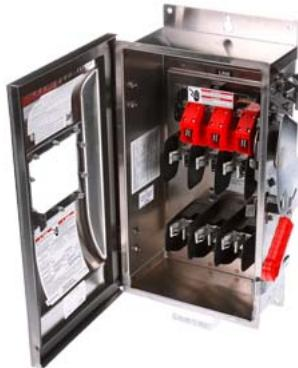
Siemens Low Voltage Circuit Protection Heavy Duty Safety Switches. Type: ENCLOSED, SAFETY SWITCH Std: CSA V. Rating: 600V A. Rating: 60A Wattage: 3W No. Of Poles: 3P F. Rating: 60Hz Action: SINGLE THROW Material: SS Enclosure: TYPE 4X. 2-3 point mounting holes. Insulation: YES O. Cycles: 10000 O. Temperature: (-20F-120F) AMBIENT TEMPERATURE Environmental Conditions: INDUSTRIAL CORROSIVE RESISTANCE
