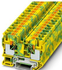
Ground terminal, number of connections: 2, connection method: Push-in connection, Rated cross section: 10 mm<sup>2</sup>, cross section: 0.5 mm<sup>2</sup> - 16 mm<sup>2</sup>, mounting type: NS 35/7,5, NS 35/15, color: green-yellow
