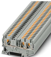
Feed-through terminal block, nom. voltage: 800 V, nominal current: 32 A, number of connections: 3, connection method: Push-in connection, Rated cross section: 4 mm<sup>2</sup>, cross section: 0.2 mm<sup>2</sup> - 6 mm<sup>2</sup>, mounting type: NS 35/7,5, NS 35/15, color: gray
