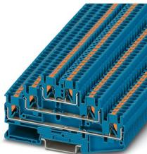
Multi-level terminal block, nom. voltage: 500 V, nominal current: 20 A, number of connections: 6, connection method: Push-in connection, 1st, 2nd and 3rd level, Rated cross section: 2.5 mm<sup>2</sup>, cross section: 0.14 mm<sup>2</sup> - 4 mm<sup>2</sup>, mounting type: NS 35/7,5, NS 35/15, color: blue
