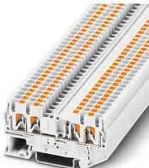
Feed-through terminal block, nom. voltage: 800 V, nominal current: 24 A, number of connections: 4, connection method: Push-in connection, Rated cross section: 2.5 mm<sup>2</sup>, cross section: 0.14 mm<sup>2</sup> - 4 mm<sup>2</sup>, mounting type: NS 35/7,5, NS 35/15, color: white
