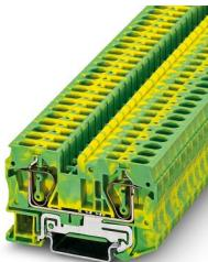
Ground terminal, number of connections: 2, connection method: Spring-cage connection, 1 level, cross section: 0.2 mm<sup>2</sup> - 10 mm<sup>2</sup>, mounting type: NS 35/7,5, NS 35/15, color: green-yellow
