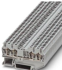
Feed-through terminal block, nom. voltage: 800 V, nominal current: 24 A, number of connections: 4, connection method: Spring-cage connection, Rated cross section: 2.5 mm<sup>2</sup>, cross section: 0.08 mm<sup>2</sup> - 4 mm<sup>2</sup>, mounting type: NS 35/7,5, NS 35/15, color: gray
