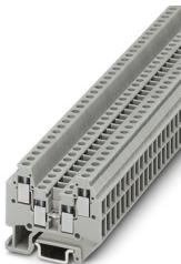
Micro terminal, nom. voltage: 400 V, nominal current: 16 A, connection method: Screw connection, 1 level, Rated cross section: 1.5 mm<sup>2</sup>, cross section: 0.14 mm<sup>2</sup> - 1.5 mm<sup>2</sup>, mounting type: NS 15, color: gray
