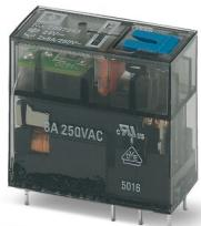
Plug-in miniature relay, with power contact, 2 changeover contacts, test button, mechanical switching position indicator, status LED, freewheeling diode, polarity A1+, A2, input voltage 24 V DC
