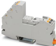
Relay base RIF-1..., for miniature power relay with 1 or 2 changeover contacts or solid-state relays of the same design, Push-in connection, plug-in option for input/interference suppression modules, for mounting on NS 35/7,5
