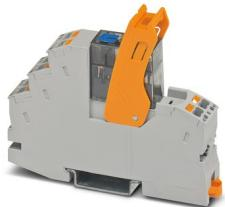
Pre-assembled relay module with Push-in connection, consisting of: relay base, relay retaining bracket, and power contact relay with test button, integrated status LED, and freewheeling diode. Contact type: 2 changeover contacts. Input voltage: 24 V DC
