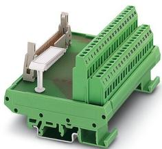
VARIOFACE module, with screw connection and flat-ribbon cable connector, for mounting on NS 32 or NS 35/7.5, with pin strip and short and long locking latches for socket strips, 26-pos.
