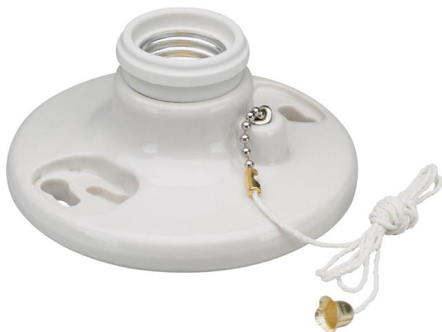
Medium base, porcelain, pullchain, 2 terminals with Tamper-Resistant-drive screws, fits 3 1/4 and 4-inch boxes, with cage neck.
