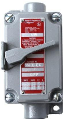
Triple-Pole, Three Phase Switch (7803) in a NEMA 7 and 9 Enclosure for Hazardous Locations. Class I - Groups C, D Class II - Groups E, F, G. 30A, 600Vs. Slotted opening on enclosures allows for lock-out, tag-out functionality.
