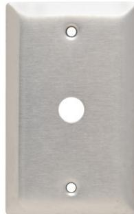
Single-Gang, Single telephone or cable outlet with removable 13/32 ft ID grommet in 17/32-inch hole. Smooth 302/304 stainless steel.
