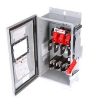
Siemens Low Voltage Circuit Protection Heavy Duty Safety Switches. Type: ENCLOSED, SAFETY SWITCH Std: CSA V. Rating: 600V A. Rating: 100A Wattage: 3W No. Of Poles: 3P F. Rating: 60Hz Action: SINGLE THROW Material: 304SS Enclosure: TYPE 12. 2-3 point mounting holes. Insulation: YES O. Cycles: 10000 O. Temperature: (-20F-120F) AMBIENT TEMPERATURE Environmental Conditions: INDUSTRIAL
