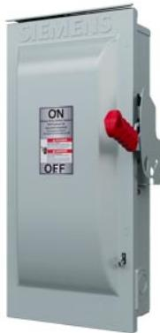
Siemens Low Voltage Circuit Protection Heavy Duty Safety Switches. Type: ENCLOSED, SAFETY SWITCH Std: CSA V. Rating: 240V A. Rating: 100A Wattage: 4W No. Of Poles: 3P F. Rating: 60Hz Action: SINGLE THROW Material: 304SS Enclosure: TYPE 3R. 2-3 point mounting holes. O. Cycles: 10000 O. Temperature: (-20F-120F) AMBIENT TEMPERATURE Environmental Conditions: OUTDOOR
