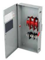
Siemens Low Voltage Circuit Protection Heavy Duty Safety Switch. 3-Pole 3-Fuse Fused in a type 3R enclosure (outdoor). Rated 600VAC (400A).
