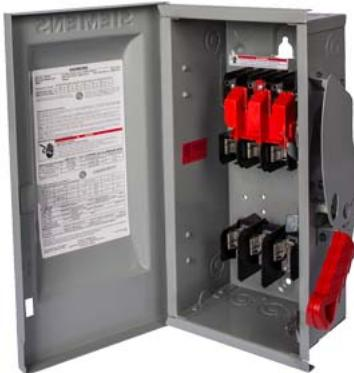
Siemens Low Voltage Circuit Protection Heavy Duty Safety Switch. 3-Pole 3-Wire Fused in a type 12 industrial enclosure. Rated 600VAC (60A). Special features: Crouse-Hinds interlocked receptacle, viewing window.
