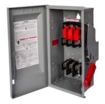
Siemens Low Voltage Circuit Protection Heavy Duty Safety Switch. 3-Pole 3-Wire Fused in a type 12 industrial enclosure. Rated 600VAC (30A). Special features: Crouse-Hinds interlocked receptacle, viewing window.
