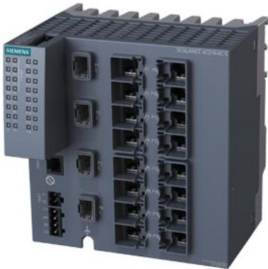
SCALANCE XC216-4C G manageable Layer 2 IE switch; IEC 62443-4-2 certified; Full gigabit; 12x 10/100/1000 Mbit/s RJ45 ports; 4x 1000 Mbit/s combo ports (either 1000 Mbit/s SFPs or 10/100/1000 Mbit/s RJ45 ports can be used); 1x console port; diagnostics LED; redundant power supply; temperature range -40 °C to +70 °C; assembly: DIN rail/S7 mounting rail/wall; redundancy functions; office features (RSTP, VLAN,...); PROFINET IO device; Ethernet/IP-compliant; C-PLUG slot;
