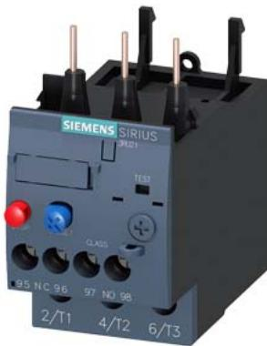
Overload relay 14...20 A Thermal For motor protection Size S0, Class 10 Contactor mounting Main circuit: Screw Auxiliary circuit: Screw Manual-Automatic-Reset
