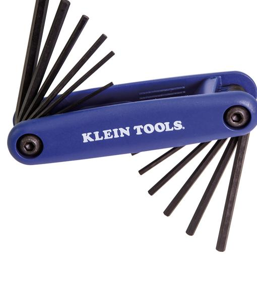
The Klein 70573 Hex Key Set ends are square-cut for a secure, full-depth fit and maximum contact with the hex socket which works to prevent slippage and stripping of the socket while in use. Sizes are: 5/64-Inch, 3/32-Inch, 7/64-Inch, 1/8-Inch, 9/64-Inch, 5/32-Inch, 1.5 mm, 2 mm, 2.5 mm, 3 mm, 4 mm, 5 mm
