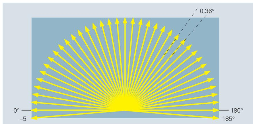
Fig. 3/53 Working area and angular resolution
