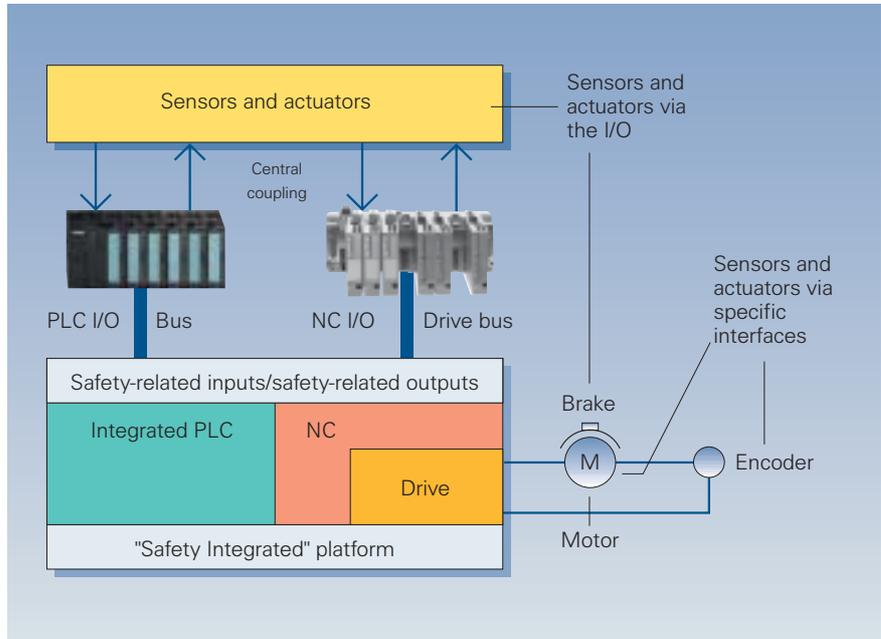
Fig. 5/16 Sensor-actuator integration via the S7 I/O and the DMP module of the NC
