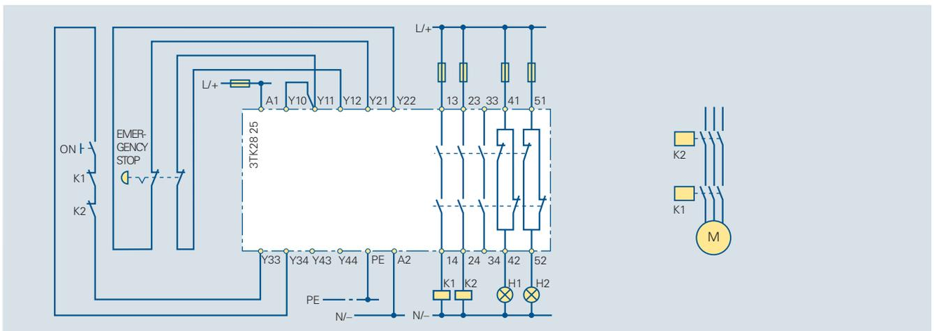
Fig. 7/14 3TK28 25 EMERGENCY STOP, Category 4, two-channel, according to EN 954-1, monitored start
