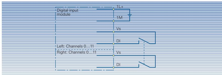
Example: Wiring schematic for a transmitter connected to an F-DI (2-from-2) through 2 channels
