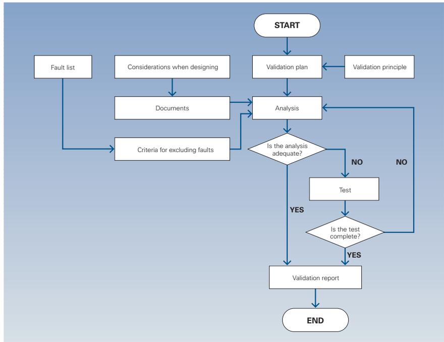
Fig. 1/8 Overview of the validation process (from prEN 954-2)
