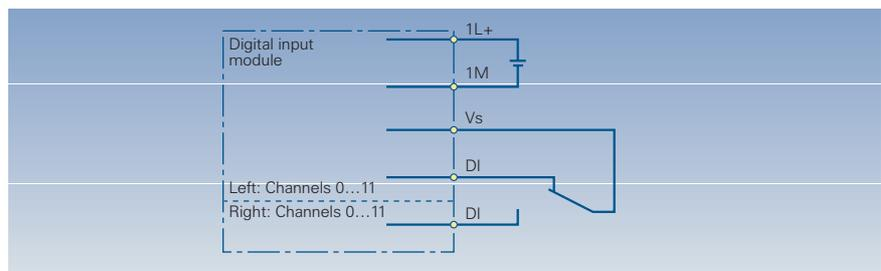
Example: Connection schematic for an anti-valent transmitter connected to an F-DI (2-from-2) through 2 channels
