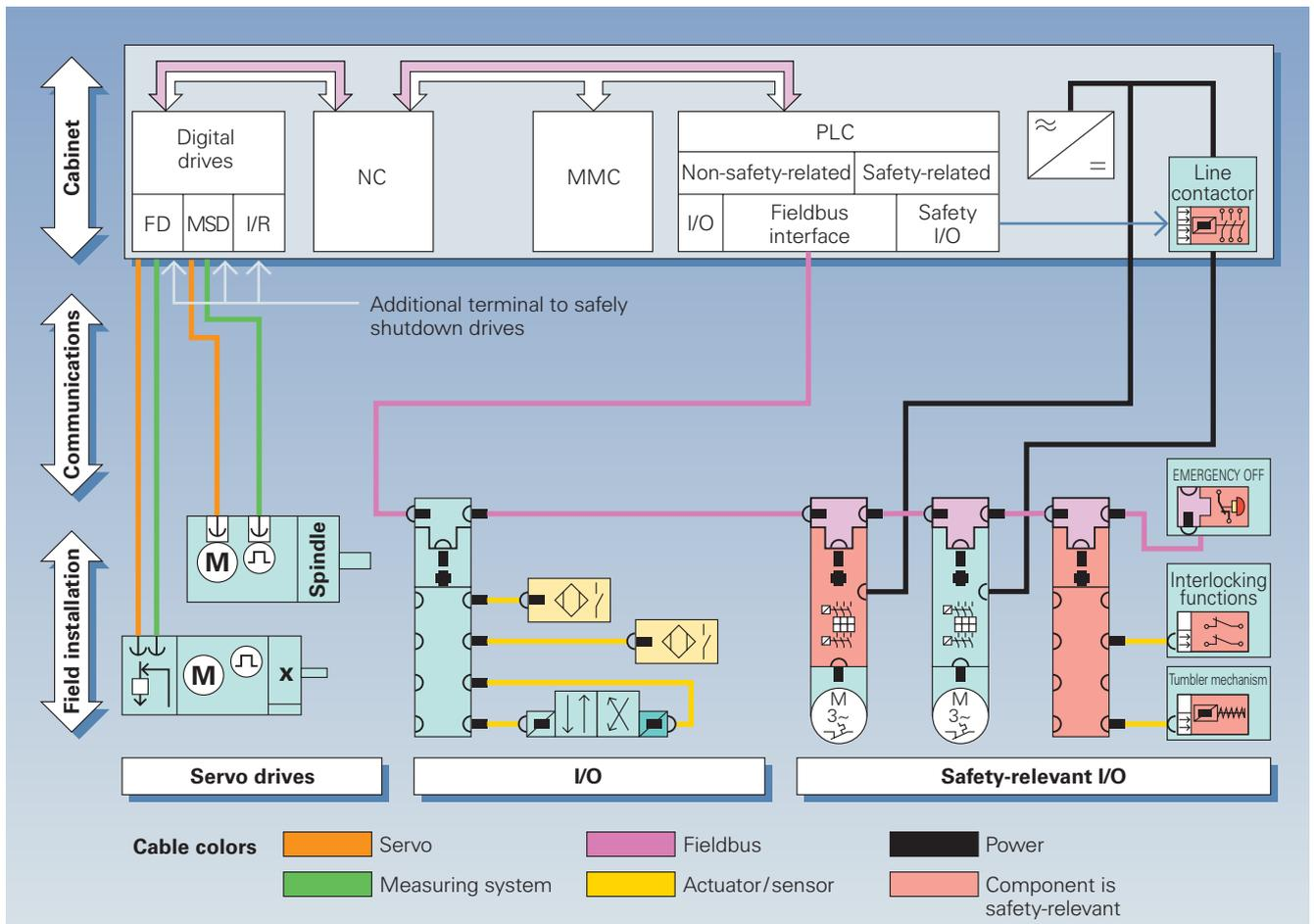
Fig. 1 Distributed and standardized installation technology in the machine environment
