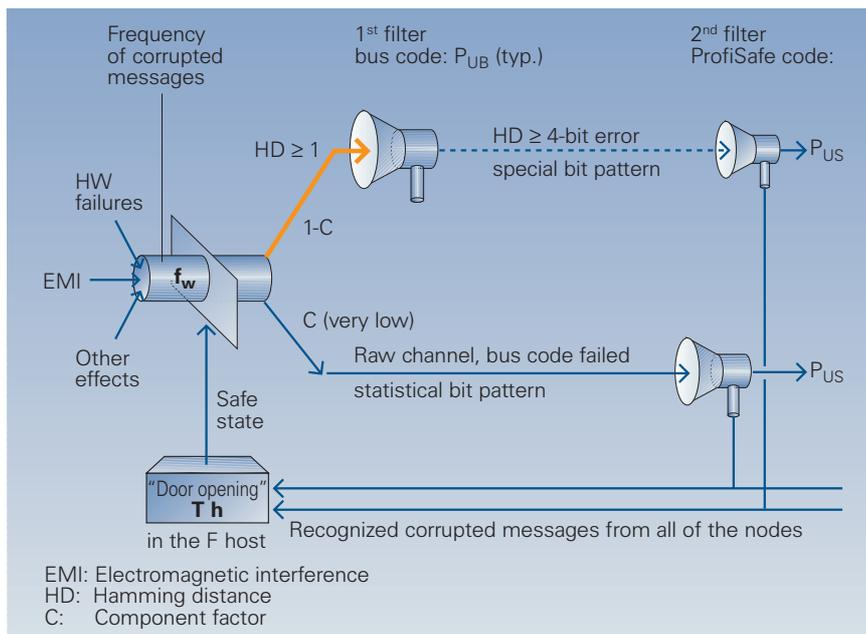
Fig. 2/6 Patented SIL monitor continually monitors the functional safety of PROFIsafe
