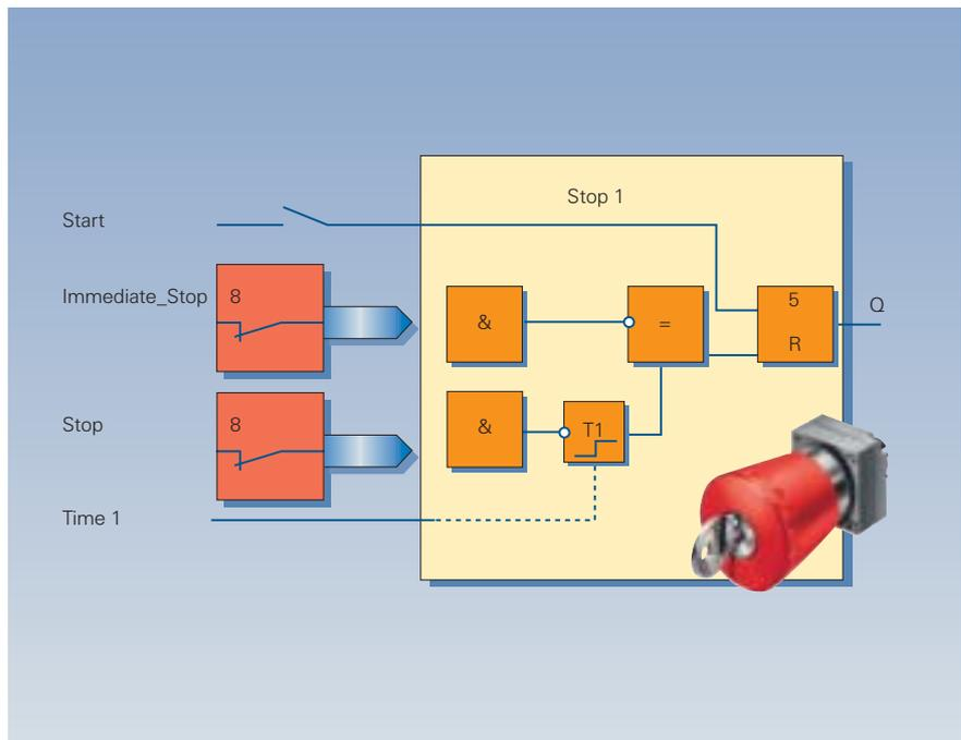
Fig. 4/9 “Emergency Stop” programming example
