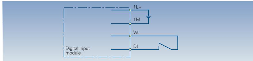
Example: Wiring schematic for a transmitter connected to an F-DI (1-from-1) through 1 channel
