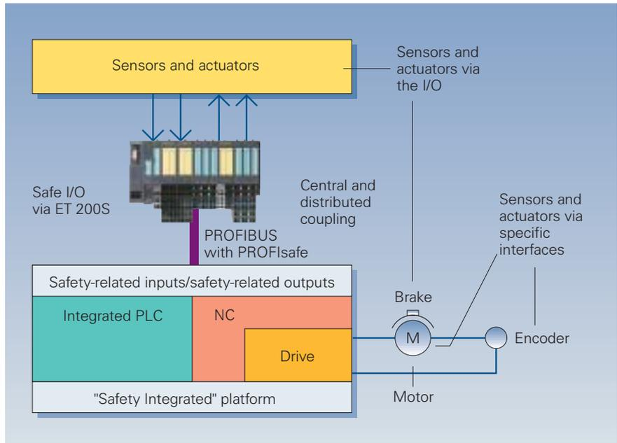
Fig. 5/17 Sensor-actuator integration via ET 200S PROFIsafe
