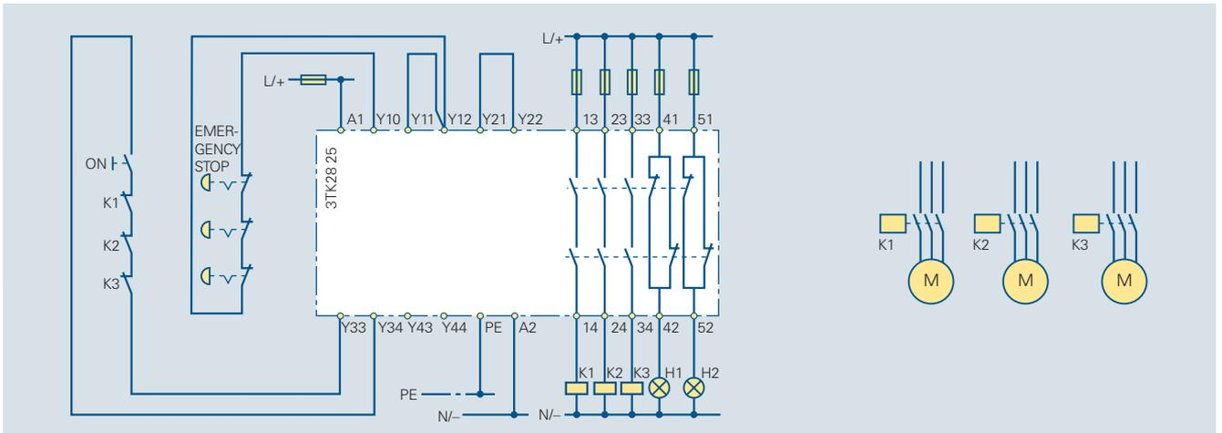
Fig. 7/13 3TK28 25 EMERGENCY STOP, Category 2, single-channel, according to EN 954-1, monitored start
