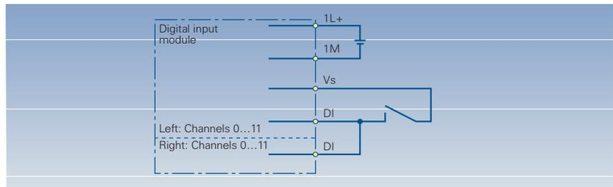
Example: Wiring schematic for a transmitter connected to an F-DI (2-from-2) through 1 channel
