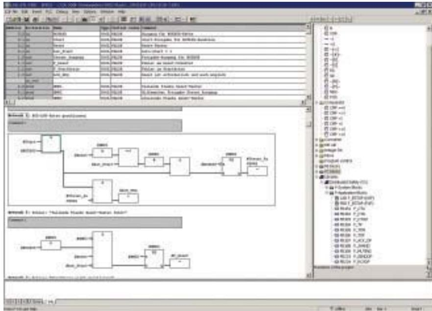
Fig. 4/8 Programming using the function block diagram (FBD)
