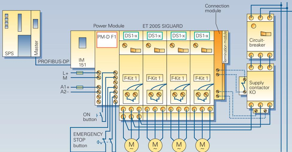
Fig. 3/68 Comparison of wiring for a conventional configuration and using ET 200S SIGUARD acc. to Category 4 in compliance with EN 954-1, EMERGENCY STOP
