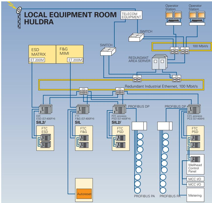
Fig. 6/8 Safety-related monitoring of an oil/gas platform with S7-400F
