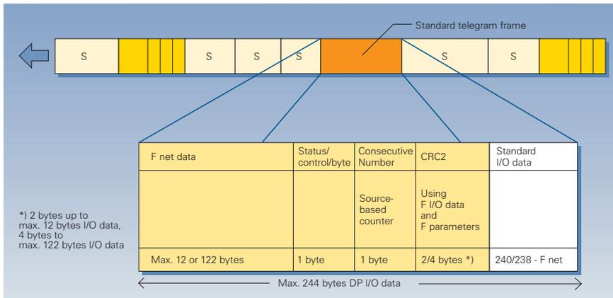
Fig. 2/5 PROFIsafe telegrams simply packaged in standard telegrams
