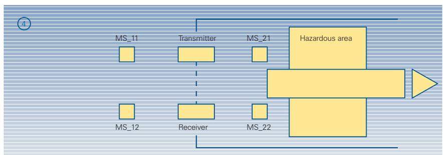
4. After one of the inputs for the muting sensors MS\_21 and MS\_22 = 0 (the product enables the sensors), the MUTING function is exited (Q = 1, MUTING = 0). The MUTING function may be active for a maximum time parameterized at the input TIME\_MAX.
