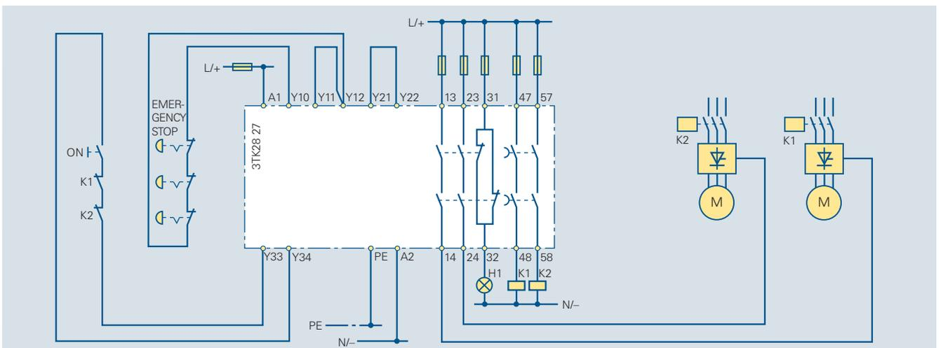
Fig. 7/15 3TK28 27 EMERGENCY STOP, Category 2, single-channel, according to EN 954-1, monitored start
