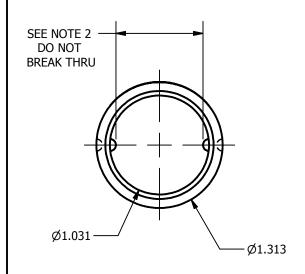
2. MUST NOT PASS Ø.958 PIN THROUGH DIMPLES
