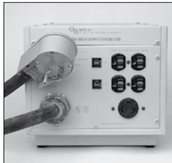
60 Hz, 2000–3000 VA, (4) 5-15R and (1) L5-30R Receptacle
