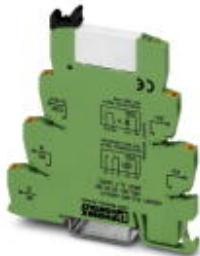
PLC-INTERFACE, consisting of PLC-BPT.../21 basic terminal block with push-in technology and plug-in miniature relay with power contact, for mounting on NS 35/7,5 DIN rails, 1 PDT, input voltage: 24 V DC
