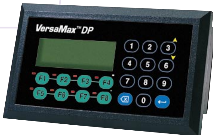
DP 85 • 8 function keys and data entry keypad • Stores 200 messages • 4 line display
