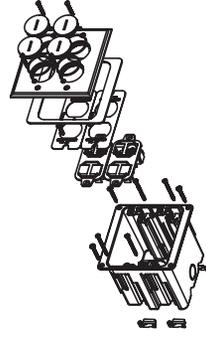
Includes dual-gang box, two 106 adapter with eight openings for communication devices, and brass cover with four screw plugs. For hole cut dimensions, see installation instructions sheet.
