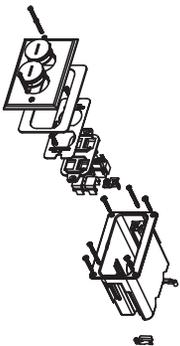
Includes single-gang box, 106 adapter with four openings for communication devices, and brass cover with two screw plugs. For hole cut dimensions, see installation instructions sheet.
