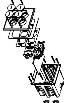
Includes dual-gang box, one 15A tamper-resistant duplex receptacle, 106 adapter with four openings for communication devices, and nickel cover with four screw plugs. For hole cut dimensions, see installation instructions sheet.
