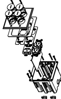
Includes dual-gang box, one 15A tamper-resistant duplex receptacle, 106 adapter with four openings for communication devices, and brass cover with four screw plugs. For hole cut dimensions, see installation instructions sheet.
