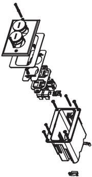
Includes single-gang box, 106 adapter with four openings for communication devices, and nickel cover with two screw plugs. For hole cut dimensions, see installation instructions sheet.
