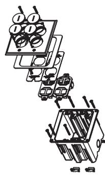
Includes dual-gang box, two 106 adapter with eight openings for communication devices, and nickel cover with four screw plugs. For hole cut dimensions, see installation instructions sheet.
