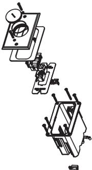
Includes single-gang box, device plate with two openings for communication devices, and nickel cover with one screw plug. For hole cut dimensions, see installation instructions sheet.
