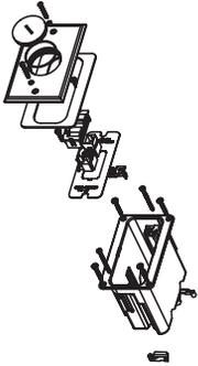
Includes single-gang box, device plate with two openings for communication devices, and brass cover with one screw plug. For hole cut dimensions, see installation instructions sheet.
