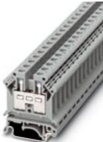
Feed-through terminal block, Connection method: Screw connection, Cross section: 0.5 mm<sup>2</sup> - 10 mm<sup>2</sup>, AWG: 20 - 8, Width: 8.2 mm, Color: gray, Mounting type: NS 35/7,5, NS 35/15
