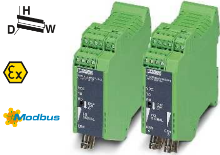
RS-485 2-wire PCF and fiberglass (multi mode)
