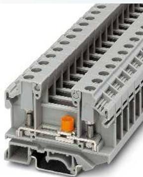
6 (6) mm 2 , 36 A, test disconnect terminal block, with test socket screws
