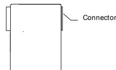
5. **Install additional modules** by mounting modules on their carriers and sliding them along the DIN rail to fully engage the connectors in the sides of the carriers.
