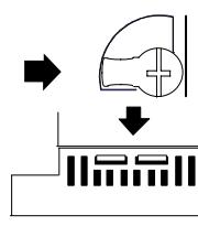
The latch on the module must be in the unlocked position.
