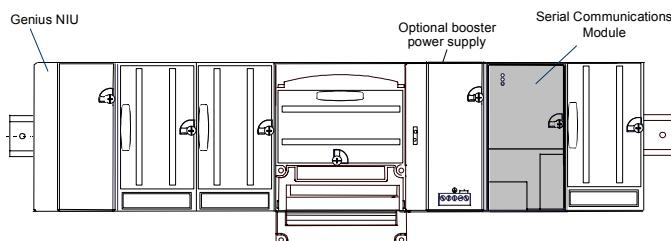
The module will support communication baud rates of 1200, 2400, 4800, 9600, and 19200, and half or full duplex operation.
