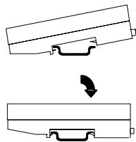
Note: Connecting carriers must be installed on the same section of 35mm x 7.5mm DIN rail.
