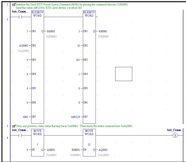
As before, to trigger the command, the sequence number, %AQ0002 must be incremented.
