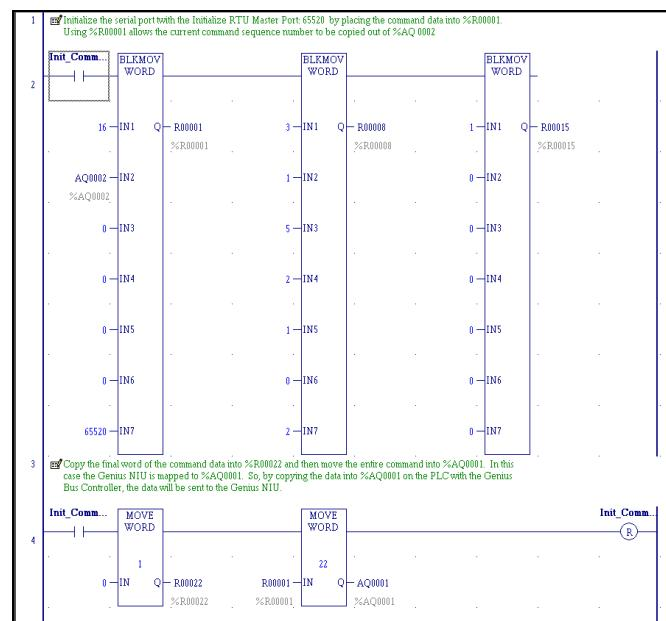
To trigger the command, the sequence number, %AQ0002 must be incremented.
