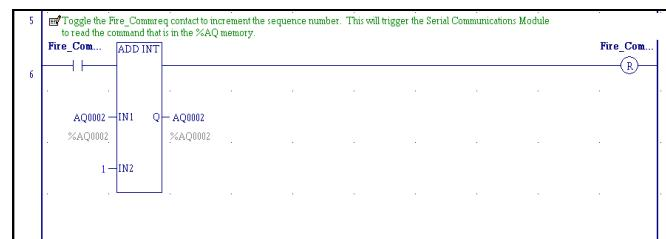
When the sequence number in %AI0002 matches the value sent in %AQ0002, it checks the command status value. If the command status value in %AI0001 is 1, the command has been successfully executed. The Serial Comm Module is configured as an RTU Master and ready to accept Modbus RTU commands.
