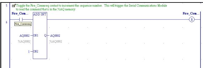
When the sequence number in %AI0002 matches the value sent in %AQ0002, it checks the command status value. If the command status value in %AI0001 is 1, the command has been successfully executed. The Serial Communications Module has successfully transmitted the Modbus RTU command to RTU Slave Device 3.
