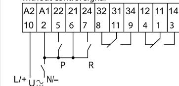
**BE:** Off-delay with control signal
