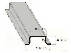
DIN Standard 75mm (symmetric Extra-Heavy-Duty "LARGE") Mounting Rail (order by part number)
